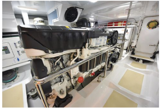
Volvo Penta D13 engines can propel the 53 to 27 knots.
